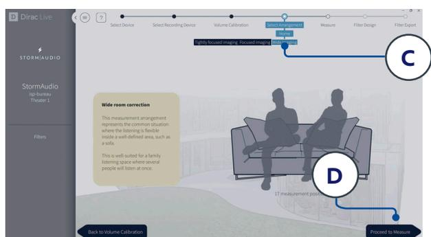
Start the measurement by pressing Proceed to Measure button (D). Keep the room silent during the process, the measurement waveform graphic is updated in real time.
