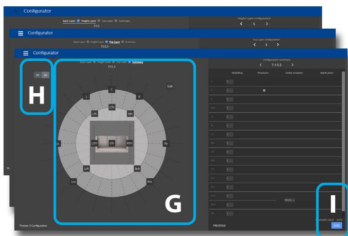
Configuration is shown. A four digits description is given following this order; "Base Layer . LFE . Height Layer . Top Layer".
